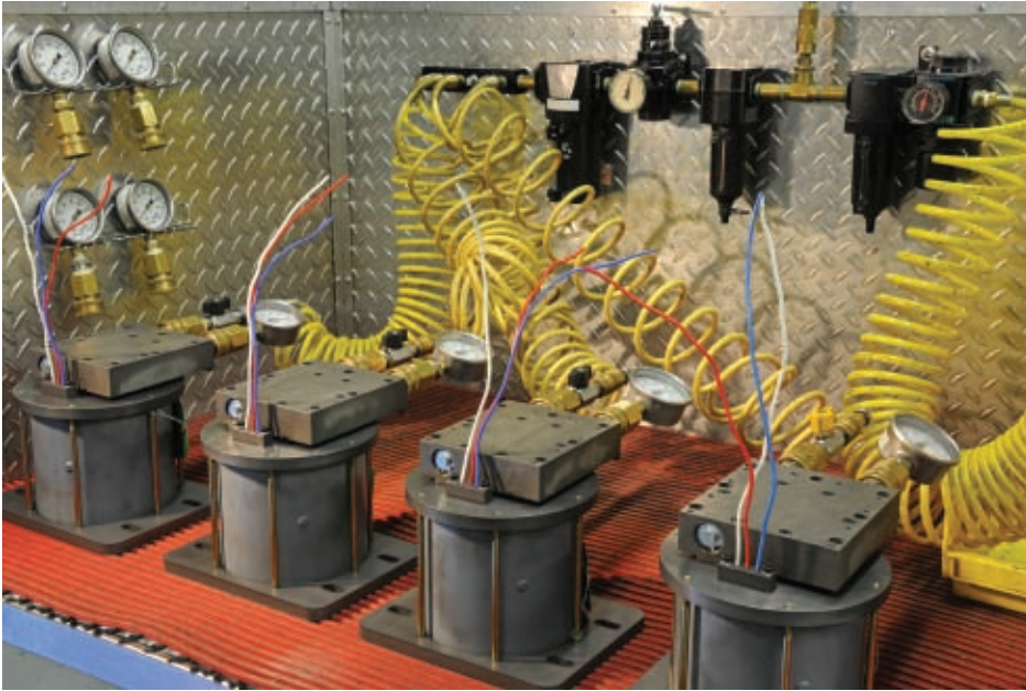
Each Paragon product is thoroughly tested in-house prior to being shipped to the customer. This test, the first of many, is designed to check all seams and welds to make sure there are no leaks.
