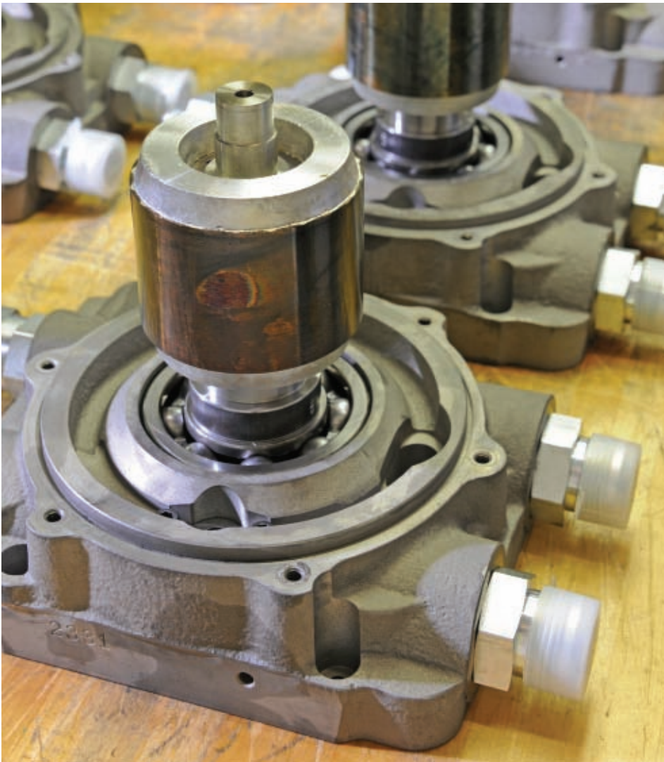
After rotors have been attached to pump brackets, they are ready for final assembly.
